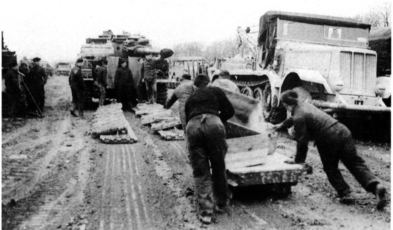
After the battalion was reconstituted in the autumn of 1943, it was transported to the Eastern Front. On 10 December 1943, the tanks changed tracks in Bialystock upon leaving the smaller European gauge railway track.
