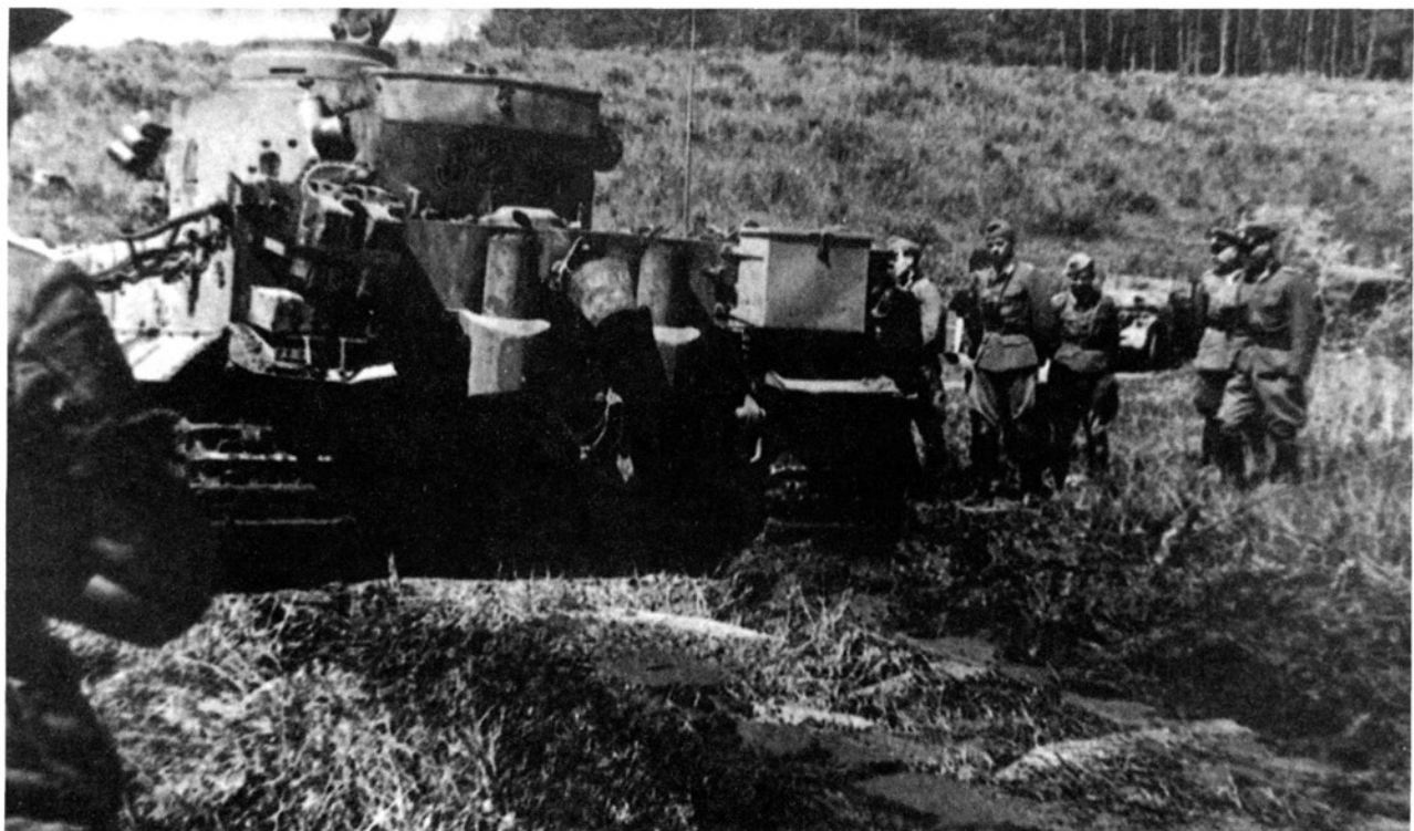
Tiger 324 nearly got bogged down. In such situations, the best course of action was for the driver to maintain as straight a course as possible and avoid applying too much power to the tracks. In no case, should the driver halt the vehicle. VON ROSEN
