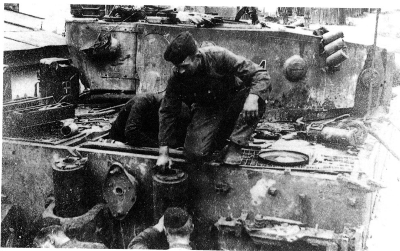
During the operational pause in preparation for the build-up to Operation "Citadel," the battalion had the opportunity to conduct repairs and maintain its vehicles. Here we see work being performed on the massive twin mufflers of the tank. HAASE
