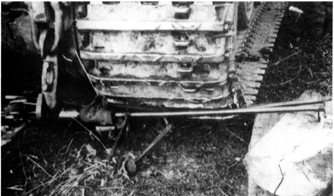
A simple way to destroyed captured enemy antitank rifles. WINKENBACH
