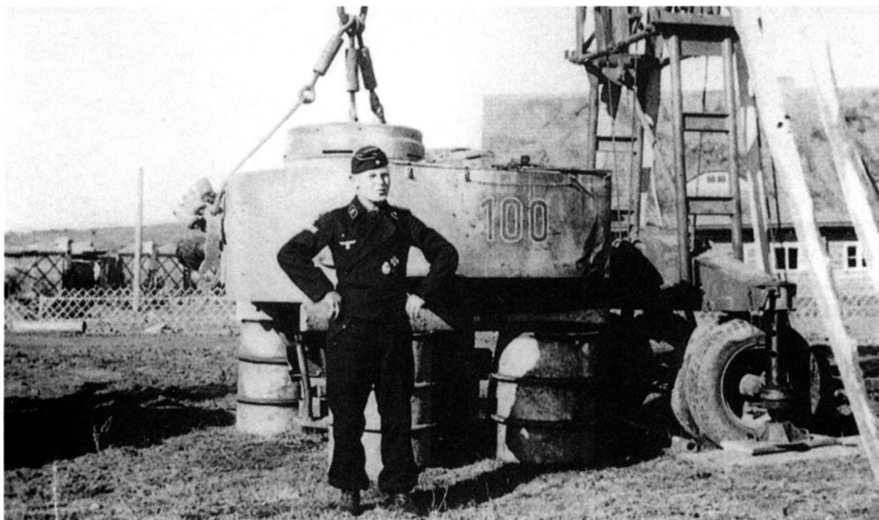
Two-hundred-liter fuel drums are used to support this turret, which has been removed from a Tiger hull. Feldwebel Stigler poses in front of Tiger 100. BOCHE
