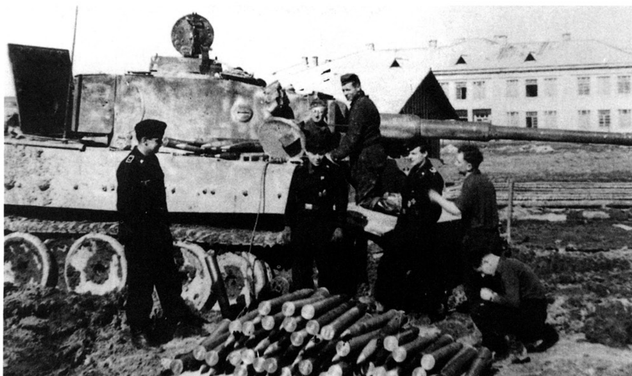
All ammunition had to be removed from a tank before any welding work could be done on the interior.
