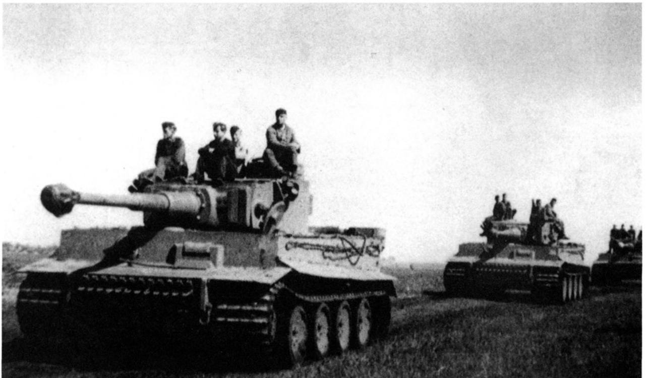
These Tigers of the 2./schwere Panzer-Abteilung 505 have an interesting field modification: They have a sun shield placed to the left of the gunner's sights. MÜNCH
