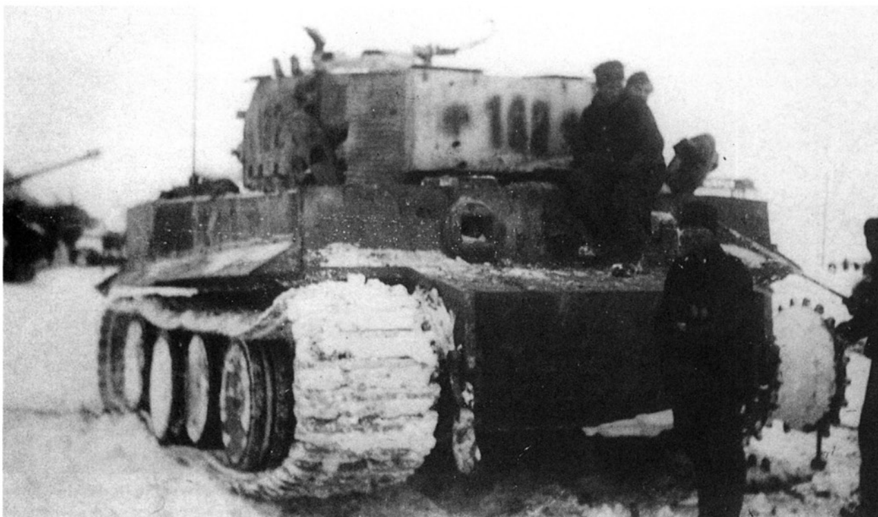
Another practice unique within schwere Panzer-Abteilung 503 was the placement of two Balkenkreuze to either side of the tank identification numeral on the turret rear stowage box. This Tiger is one of the tanks delivered later and has had Zimmerit applied to it as well as winter camouflage.
