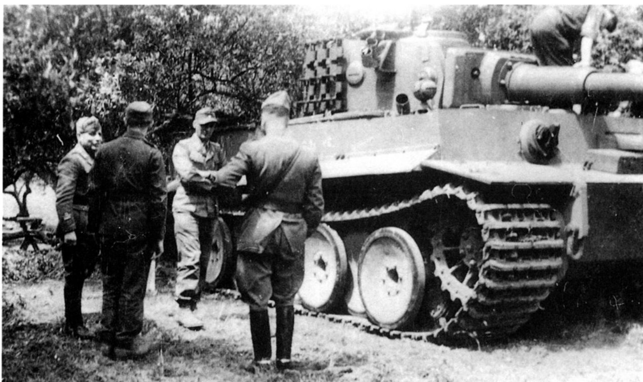
The reconfigured company was visited by high-ranking Italian officers, still “faithful” allies of the Wehrmacht. Another distinguishing feature of the new tanks is the addition of track links to the turret sides.
