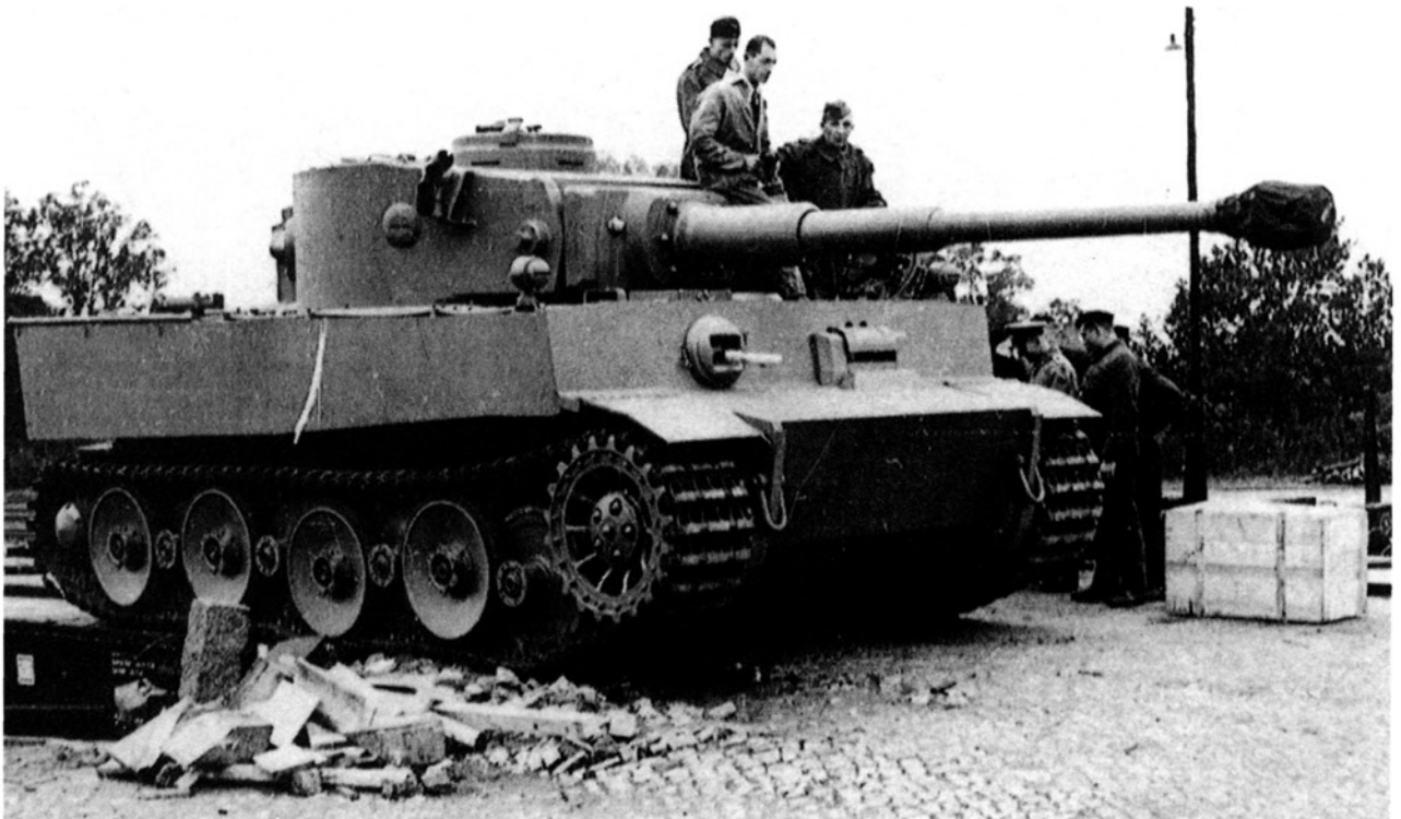
The crate in front of the crew contains the basic issue items that also arrived with the tank. The attachments for the deep-water wading kit can be seen on both sides of the hull machine-gun ball mount. Later production tanks were not fitted with these. These early tanks still lack the fixtures for mounting the track mudguards.
