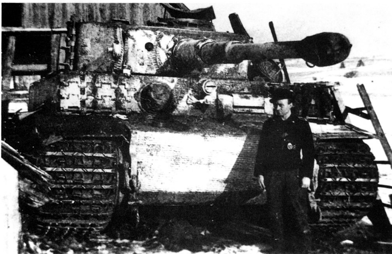
During the hard fighting in the Courland Pocket, even more armor protection was welded to the turret sides.
