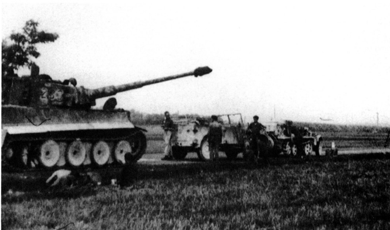
Tiger 233 during a rest halt on a road march. The maintenance contact team stands by in case any problems develop. The old-style suspension (rubber-rimmed roadwheels) indicates that this Tiger had been received from schwere Panzer-Abteilung 503. RIETH
