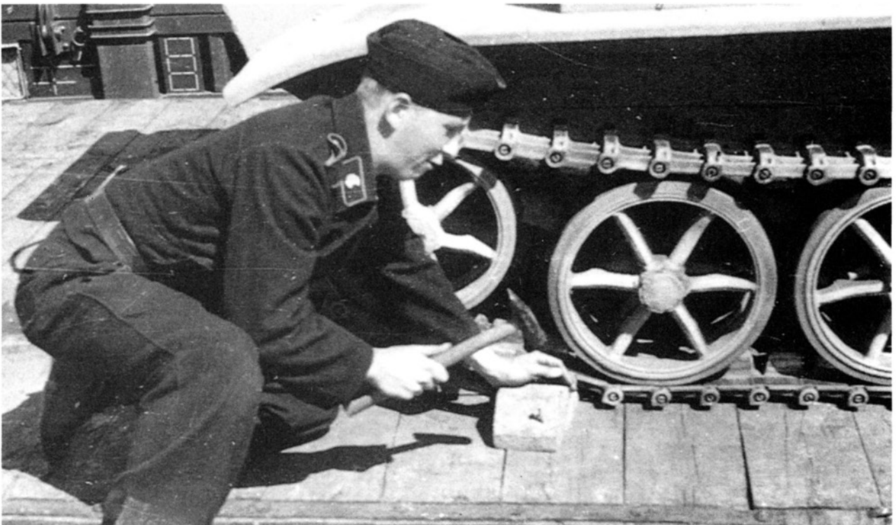
The lightweight Borgward IV had to be secured very carefully with track blocks. SUSENBETH
