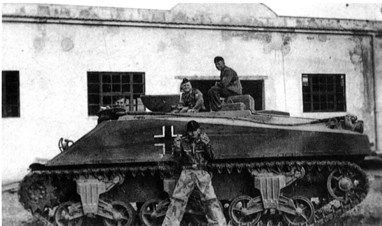
Several capture Shermans were used without their turrets as armored recovery vehicles. KETTNAKER
