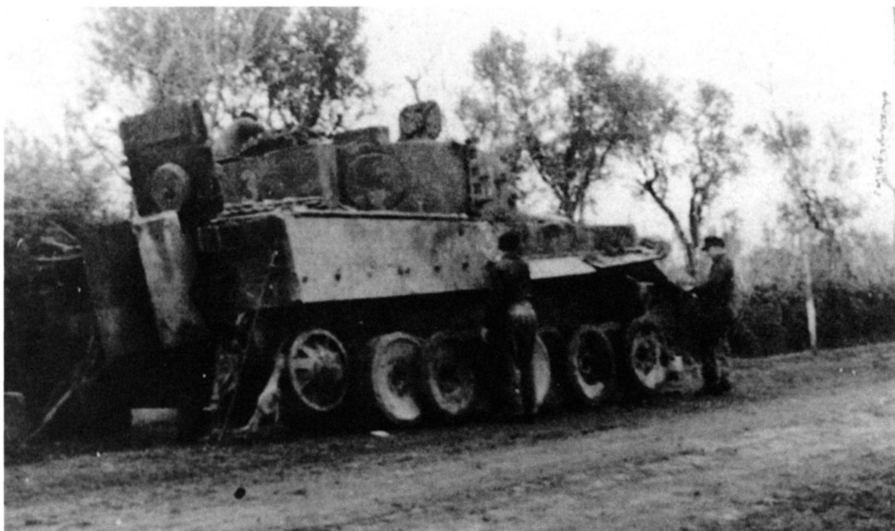
This Tiger of the 3./schwere Panzer-Abteilung 508 broke down on 13 February 1944 after its drive sprocket was damaged.
