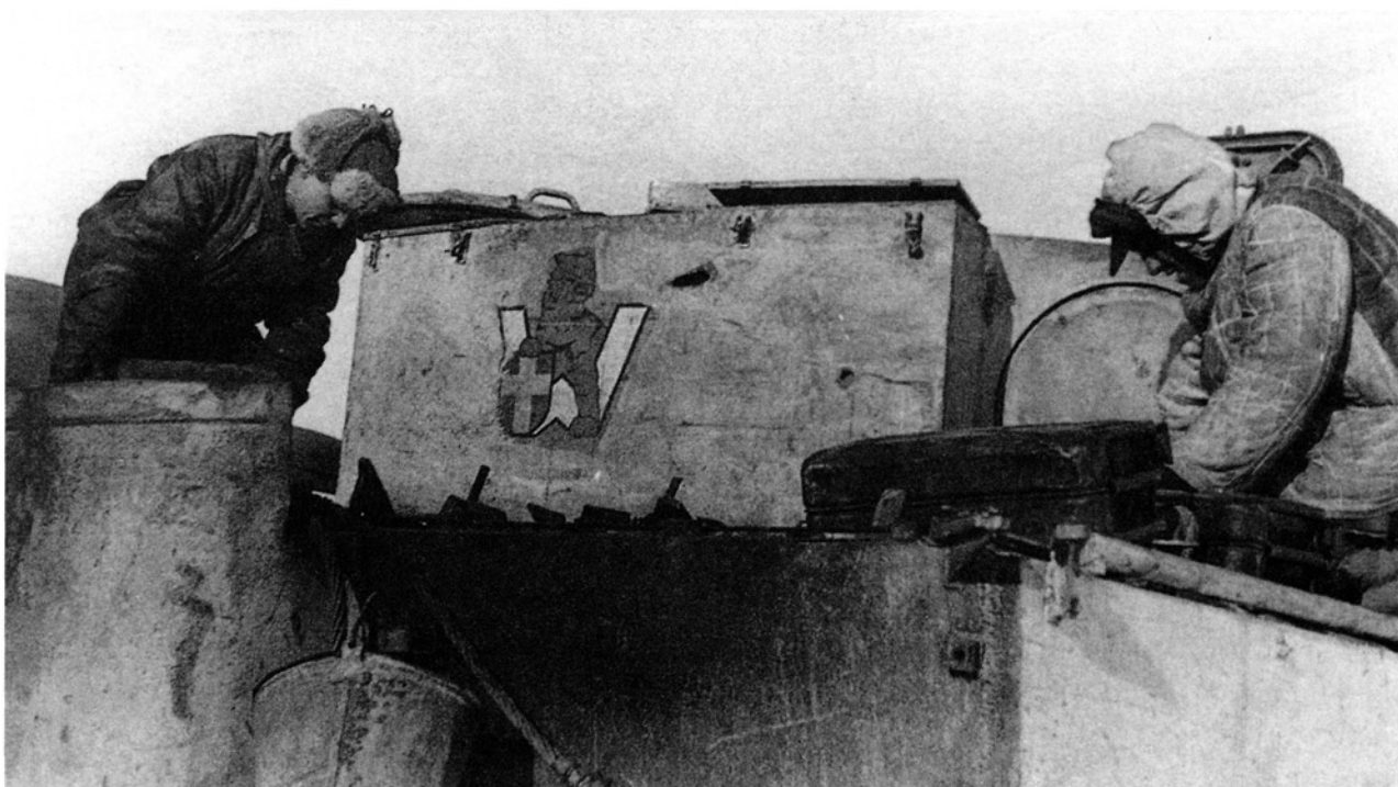
The formation insignia for schwere Panzer-Abteilung 506 was painted on the rear stowage box on the turret. The "W" was also painted in the company color; in this instance, it was white for the 1./schwere Panzer-Abteilung 506.
