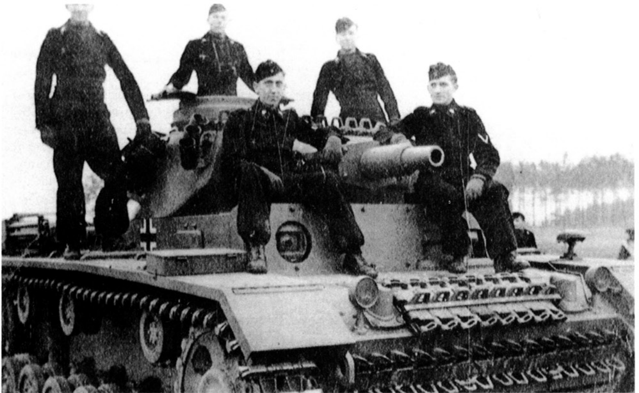
Due to the low production rate of the Tigers, the battalion was also issued with the Panzer III, Ausführung N with the short-barreled 7.5-centimeter main gun.
