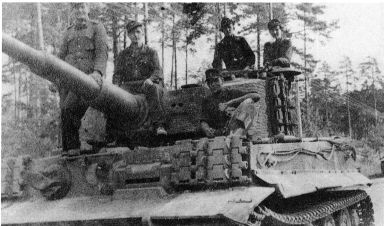
The tanks were also outfitted with additional track links on the front bow. HÜPFL
