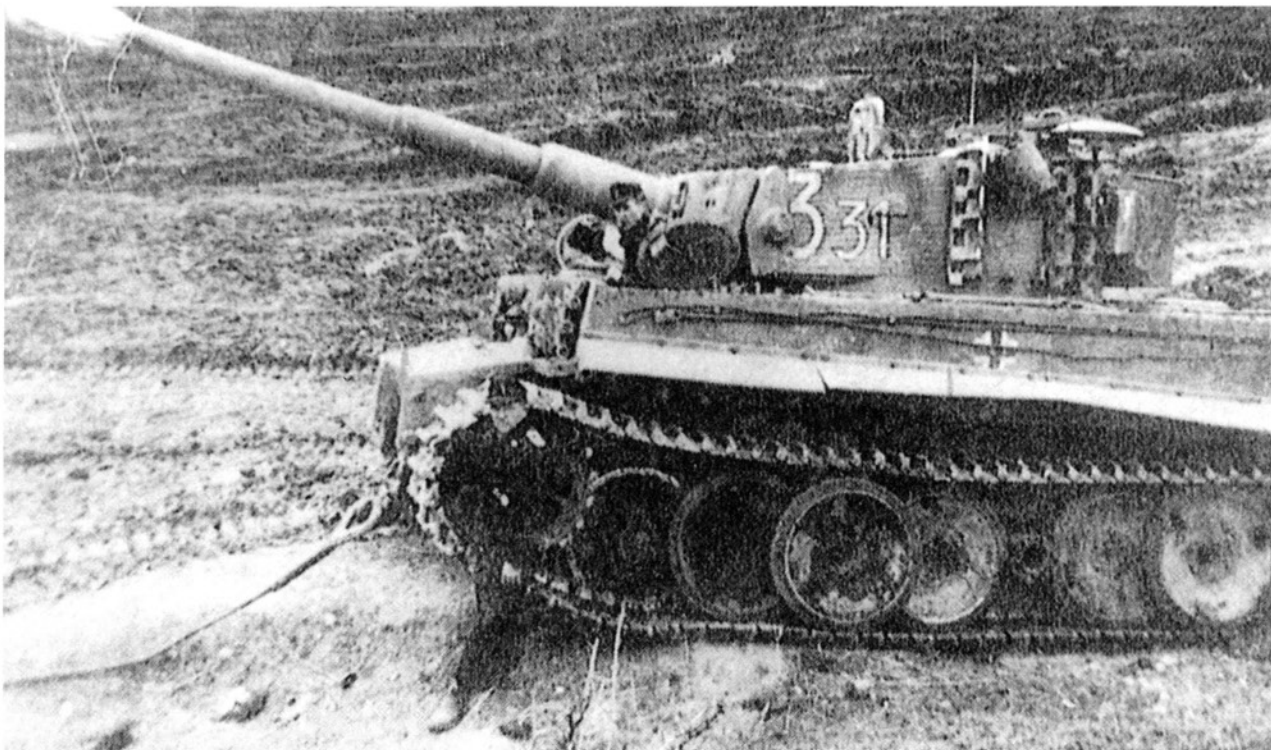
Tiger 331 of Oberfeldwebel Diez hit a mine and was immobilized. In this photograph, it has been prepared for recovery. SCHNEIDER
