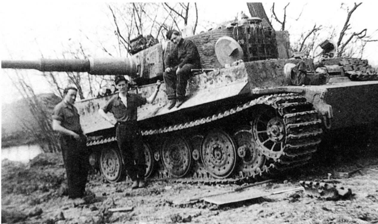
On 14 April 1944, six new tanks arrived at Zloczow. This was the latest version of the tank, which featured steel-rimmed roadwheels.
