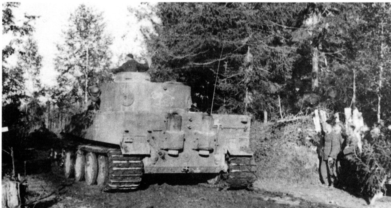
These early Tigers lacked the rear stowage boxes and featured a large mammoth where they would later be located. The exhaust stacks of the early Tigers still had not been fitted with protective metal-shield covers.
