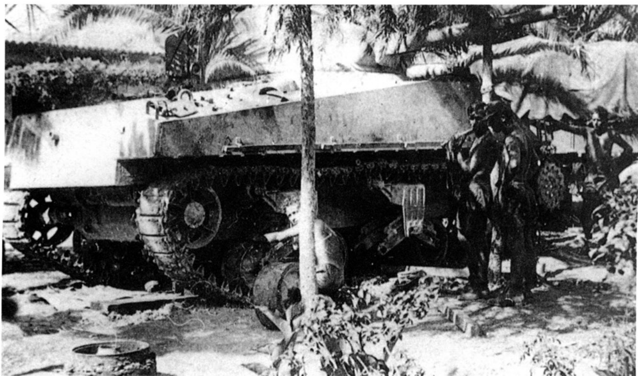
The company used a captured Sherman tank as a recovery vehicle, until it also broke down and needed new roadwheels—an item not in the German supply system! GOLDSCHMIDT
