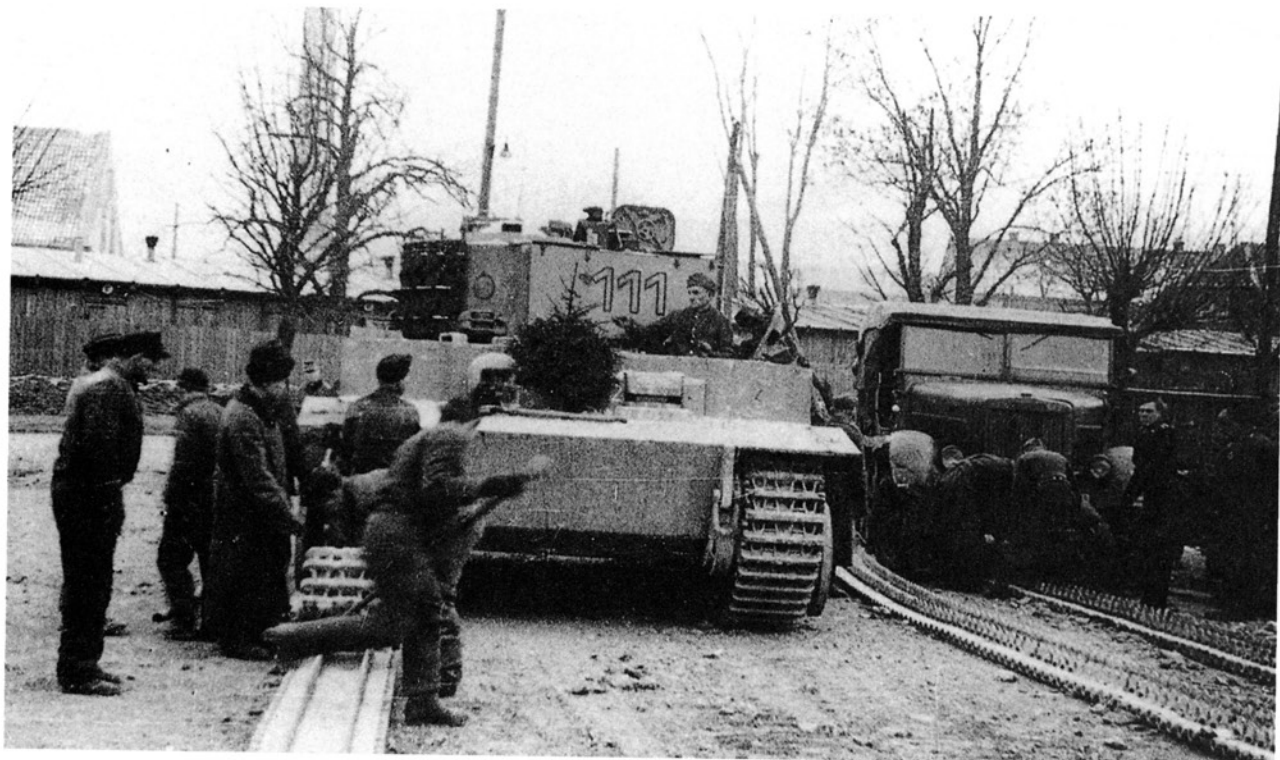
Tiger 111 has just backed off its transportation track, and the crew has started to roll it together. Once out of the way, the combat track will be placed in front of the tank, so it can then be put on the running gear. Note that the outer roadwheels have already been attached.
