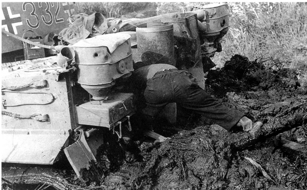
It is not easy to attach the tow cables, when the tow hooks are buried in mud.
