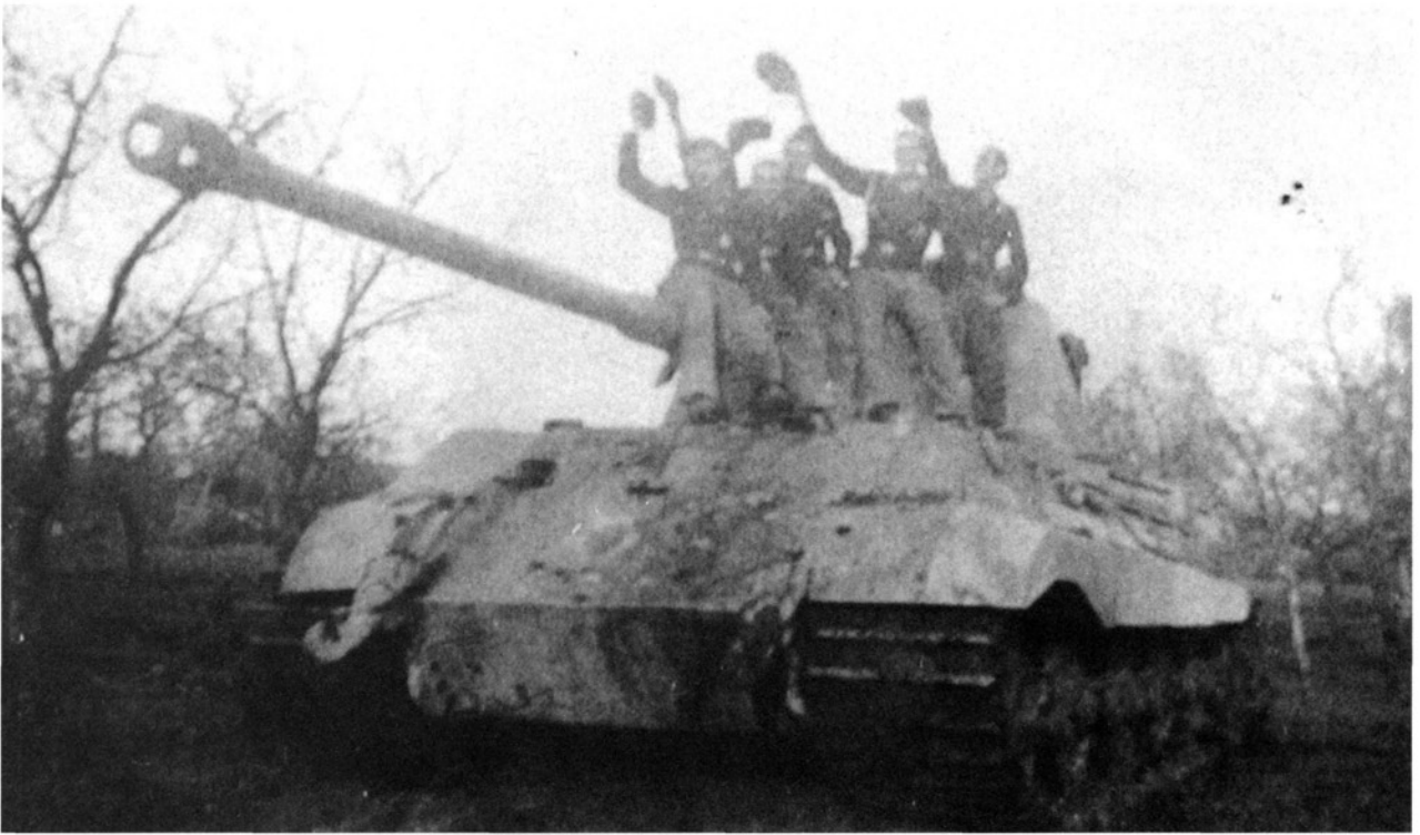
To facilitate recovery during combat operations, tow cables were frequently attached to tow hooks in advance. Or, as can be seen here, two sets of tow hooks were attached.
