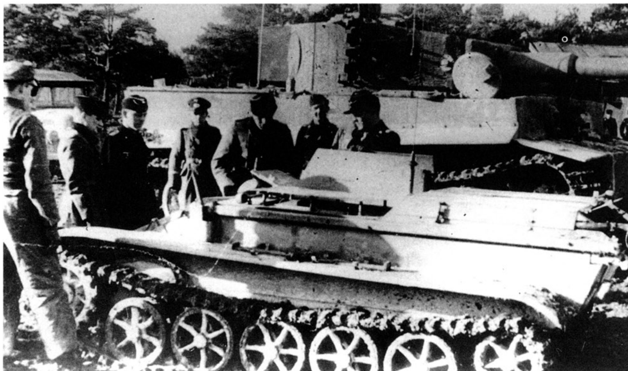
Major Hudel (right) and officers of the battalion have a first look at the Borgward IV. The additional radio guidance antenna for the demolition carrier can be seen on the right-hand turret side of the Tiger. HERWIG
