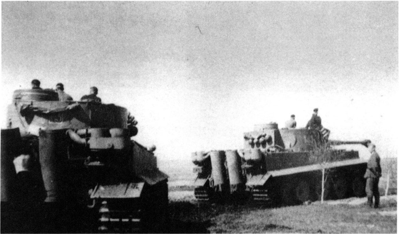
All of the Tigers have the Feifel air-filtering system, as seen here on Tigers 143 and 113. A swastika flag has been attached to the turret rear stowage boxes as an air-recognition panel. MÜNCH
