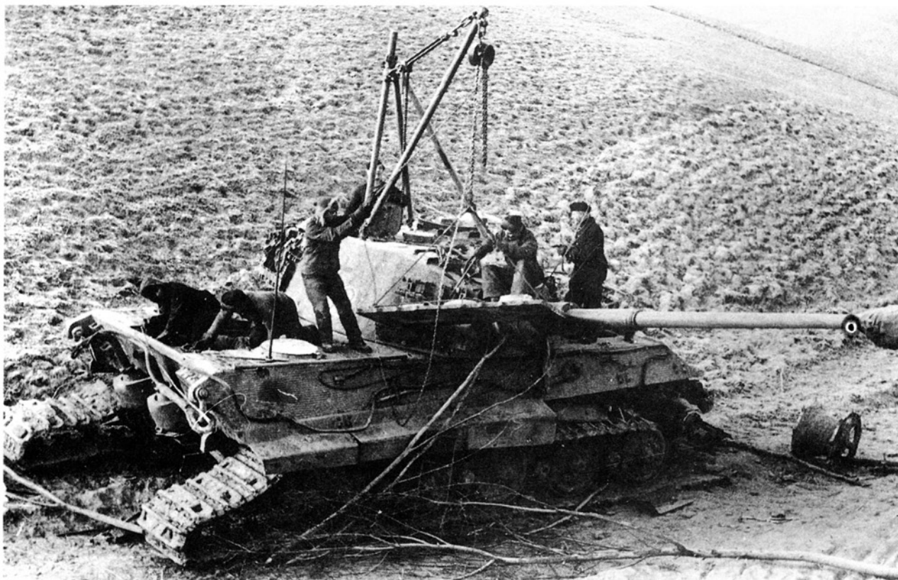
An impressive picture of field maintenance being performed in harsh winter conditions. Later model Tiger Is and all Tiger IIs were fitted with three mounting brackets on the turret roof, which allowed the set up of this useful hoist. The crew did not need an external crane for then lifting the heavy engine access plate off the deck in order to gain access to the engine compartment. BLASCHKA
