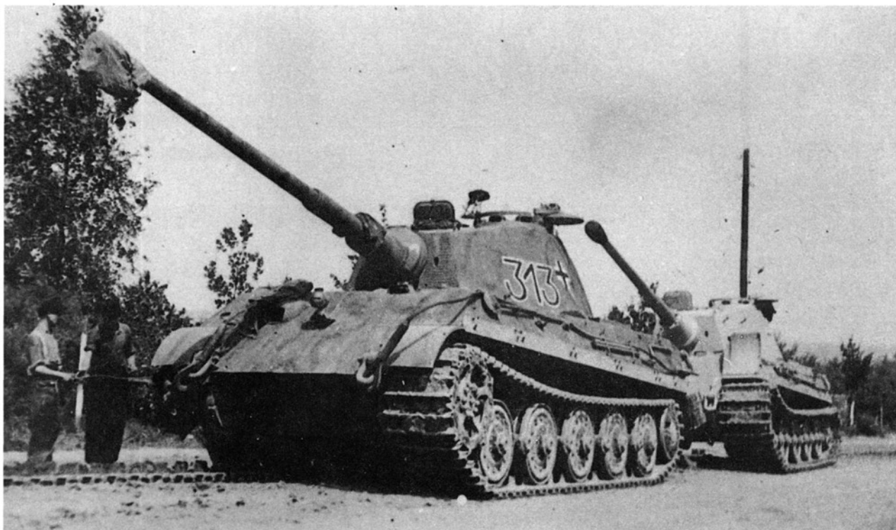
This Tiger II, also with the Zimmerit antimagnetic paste, had large turret identification numerals, which were painted in red with a white outline.
