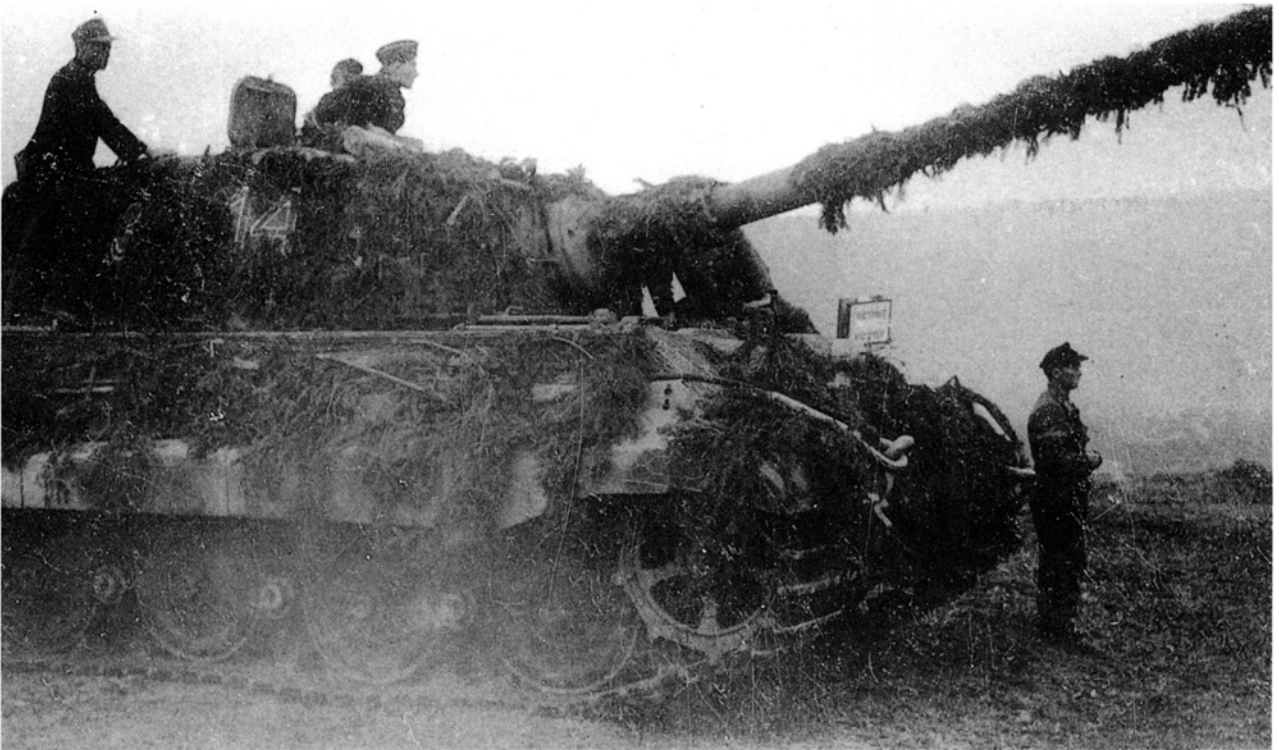
When the battalion received the Tiger II, the consecutive system of numbering was retained, but a numeral indicating the company was added. It was placed forward of the central Balkenkreuz. Tiger 3+14 had black numerals outlined in yellow. VON RÖMER
