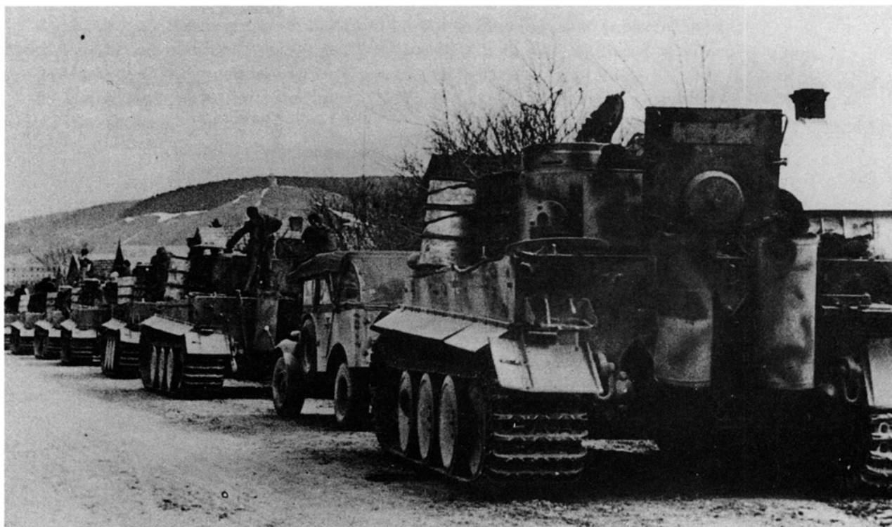
Long-distance movements required additional logistical preparations for the “thirsty” Tigers. This column from schwere Panzer-Abteilung 506 is seen during a maintenance halt. The engine access panel on the tank in the foreground has been opened to allow the engine to cool faster. Each tank has been provided with two 200-liter fuel drums.
