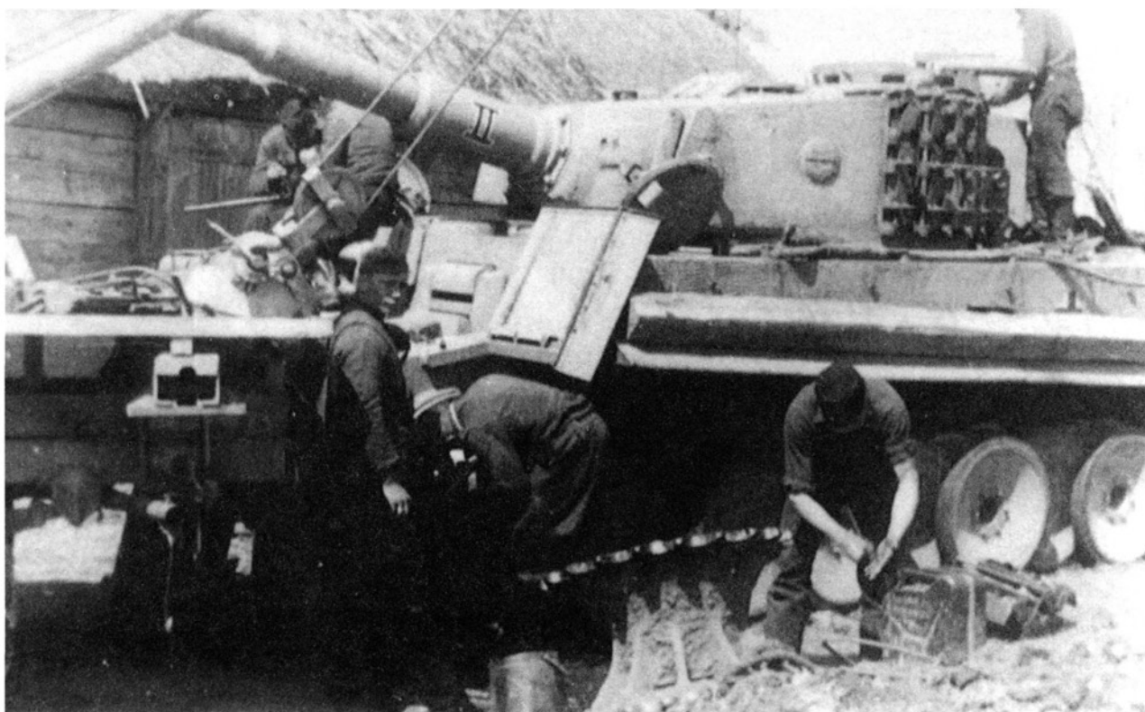
This battalion headquarters tank—Tiger II—was one of the new tanks delivered in September 1943 and features the later-style tank commander’s cupola.
