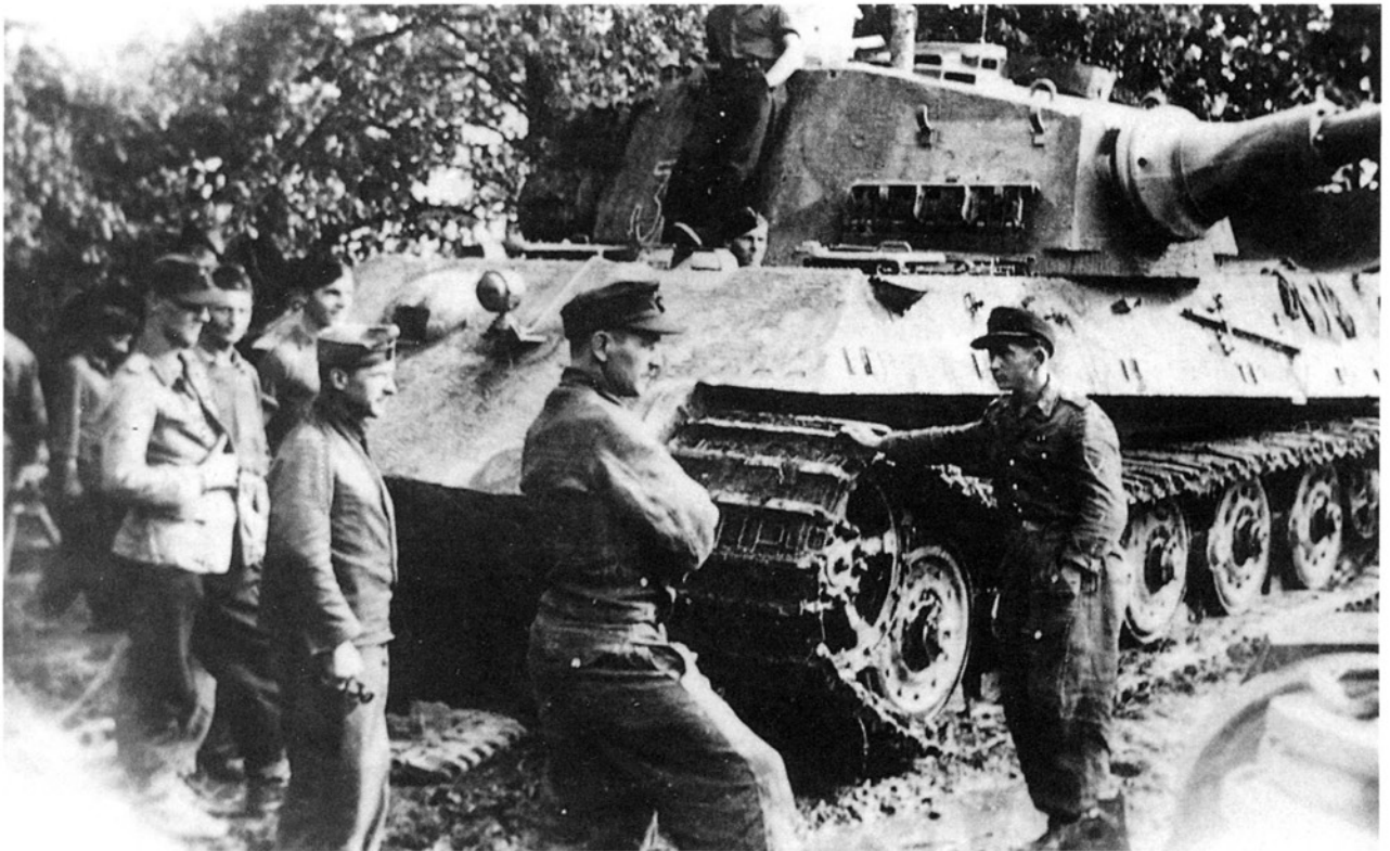
Once issued its new tanks, the battalion was redeployed to the Eastern Front, where it arrived in the Kielce Sector. The crew has apparently just finished a track repair by using one of the spare track blocks on the turret side.
