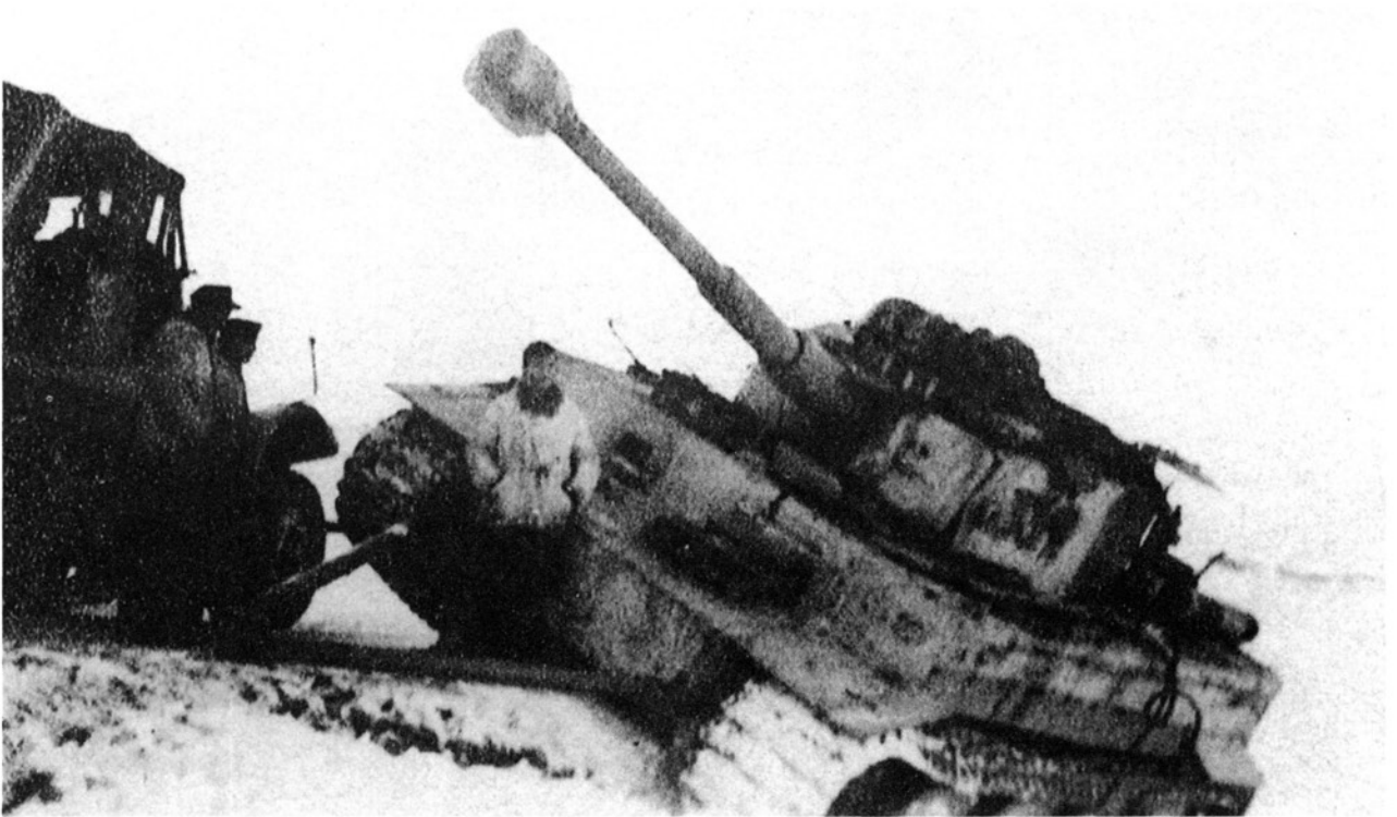
Tiger 301 has become stuck and needs assistance in being recovered in the form of an 18-ton prime mover. The tow bar has already been attached. ZORN
