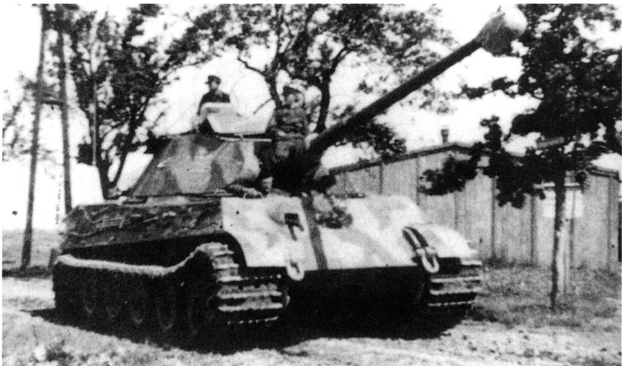
Tiger 114 has removed its track mudguards prior to changing over to the rail transportation tracks. FIEDLER
