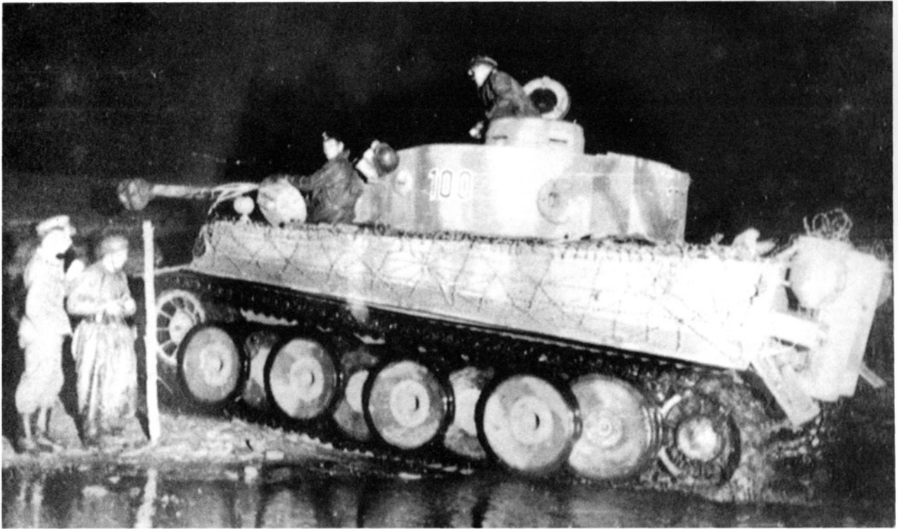
Prior to Operation "Citadel," the tanks were protected by barbed wire on all sides of the vehicle. This was designed to discourage enemy tank hunter/killer teams from climbing on the vehicles.
