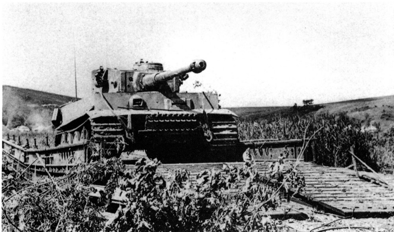
Tiger 222 crosses the engineer bridge. Ramps have been placed at both ends of the bridge to facilitate its crossing.
